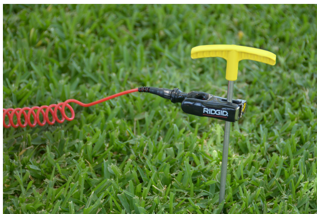
Figure 6 – Cable Lead attached to a Ground Stake
