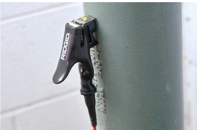
Figure 9 – Using the magnet embedded in the Cable Lead to connect to the target
