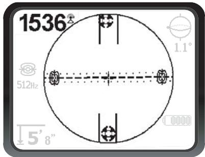
**Figure 23 – Sonde Locate: Equator**
