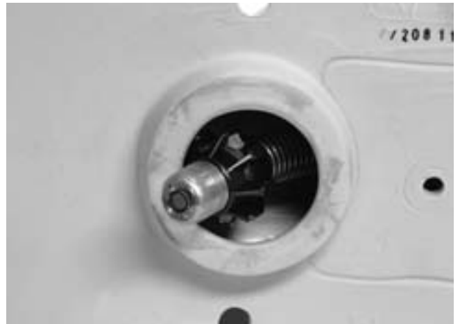
Figure 21 – Camera Head with Ball Guide in Turn
