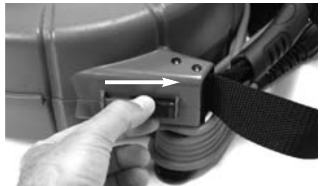
Figure 4 – Unlatching the microDrain Reel Case
