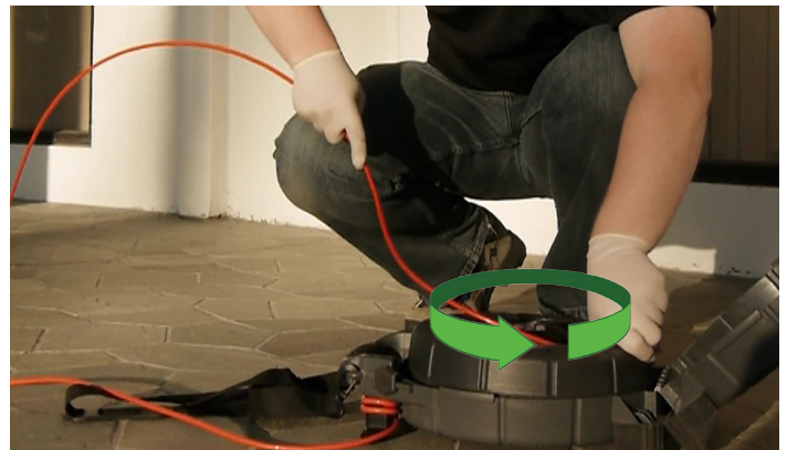
Figure 4 – Guiding the push cable into the drum
