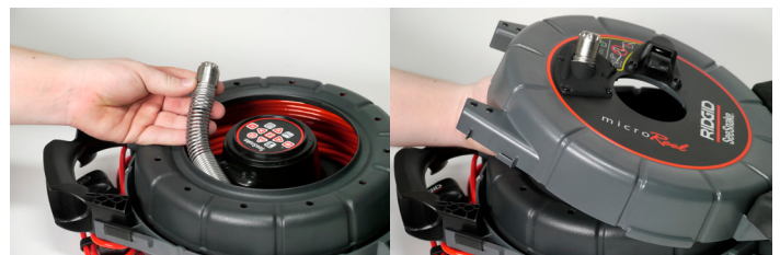
Figure 5 – Routing the camera head
