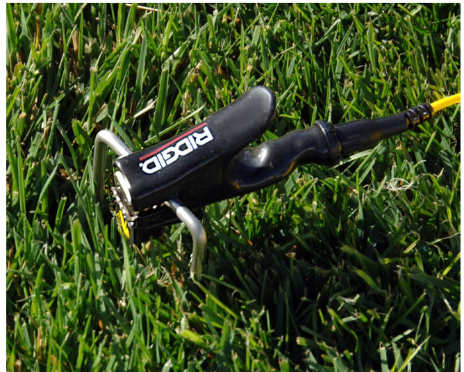
Figure 5 – Connecting the ST-305 Ground Stake
