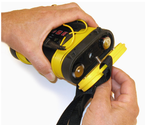
Figure 4 – Removing the Battery Cover
