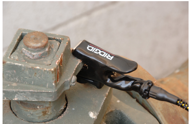
Figure 6 – Connecting the ST-305 using the clip
