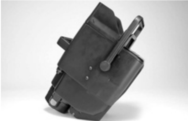
Figure 11 – Monitor Pack Tilted Using Rear Supports
