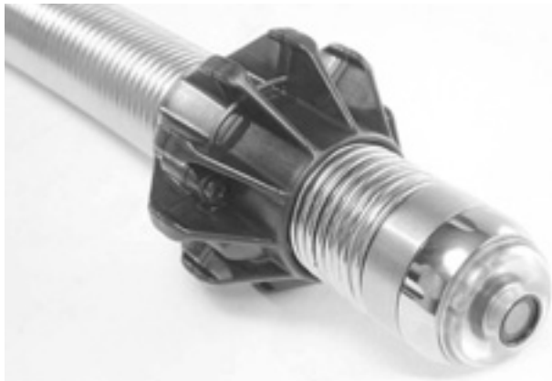
Figure 27 – Slide Ball Guide over spring and push Retaining Rings down to lock the guides in place.
