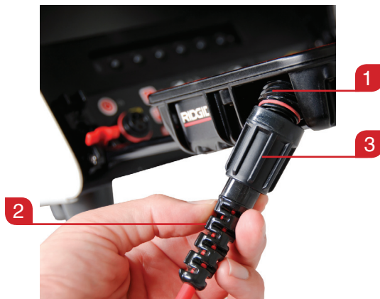
Figure 8 – Connecting SeeSnake System Cable to CS1000 System Connection
