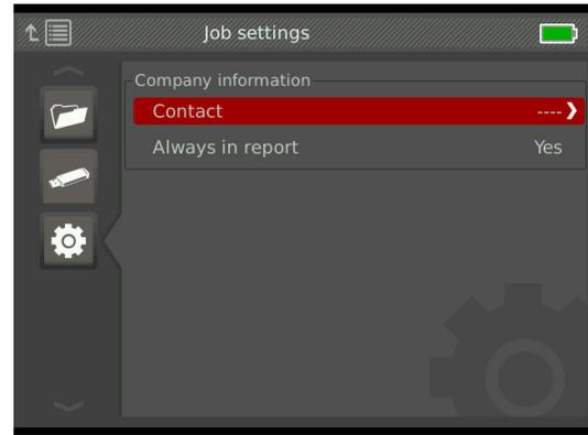
2. Highlight the field you want to edit and press the Select key
