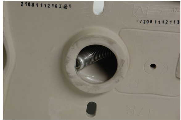
Figure 17 – Camera Head Blocked in Turn
