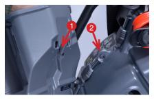
3. To secure the stow bin, pull and snap the front and back hooks into the closest groove on the rM200 case.
