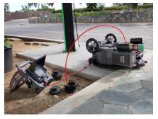
Use the pull handle as a kick stand when performing an inspection on a rooftop, hillside, or in a location that requires overhead entrv.
