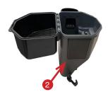
2. Install the can holder on the other side of the stow bin and screw the replacement plate into place.
