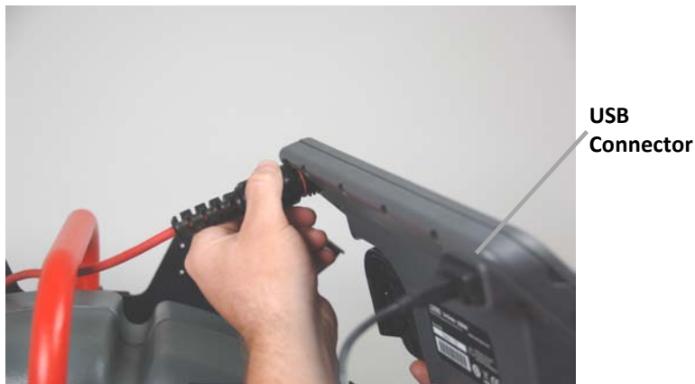
Figure 11: Attaching the SeeSnake System Cable
