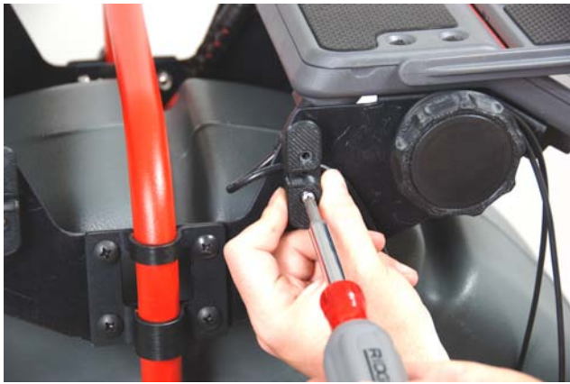
Figure 15: Mounting the Cord-Wrap (Note USB Cable captured under Cord-Wrap)
