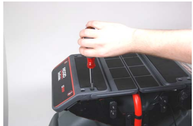
Figure 14: Mounting the Left-Hand Platform
