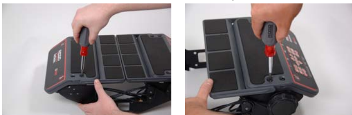
Figure 7: Removing the Platform Screws (SeeSnake Standard)
