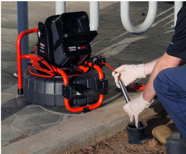
While the CS6Pak can connect to any SeeSnake camera reel with the SeeSnake system cable, it conveniently mounts on the docking system on the SeeSnake Compact2 for viewing ease, quick setup, and transport.
