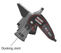
Center the CS6x Versa over the docking fins and align the docking joints with the joint sockets.
