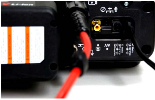
Figure 8: Connected External Power Supply
