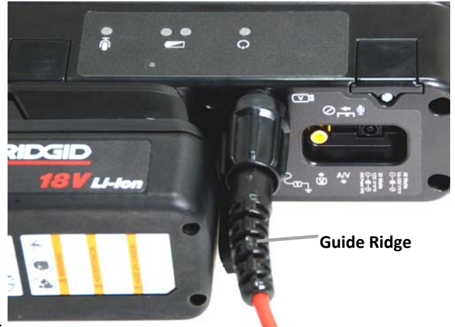
Figure 4: Connecting System Plug to DVDPak System Connector
