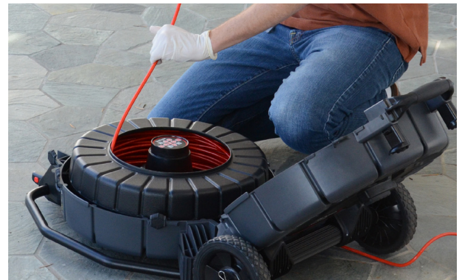
Figure 15 – Guiding the push cable into the drum
