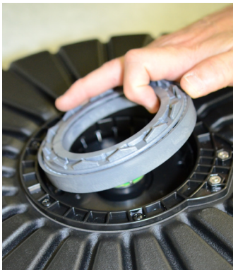
Figure 13 – Replace old bearing ring with new bearing ring.
