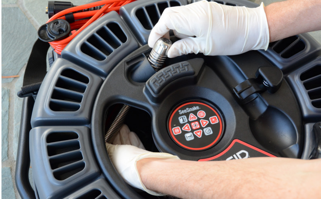
Figure 12 – Route camera head through camera access opening.
