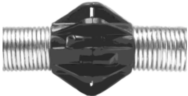
Figure 24 – Centering guides improve vision by allowing the camera to see an equal amount of pipe wall in all directions and by raising the camera out of sludge. They also reduce wear on the LED window.
