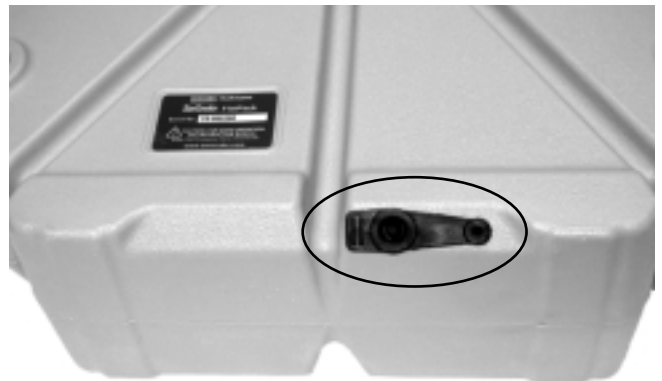
Figure 28 – Open Rubber Plug to Drain Water
