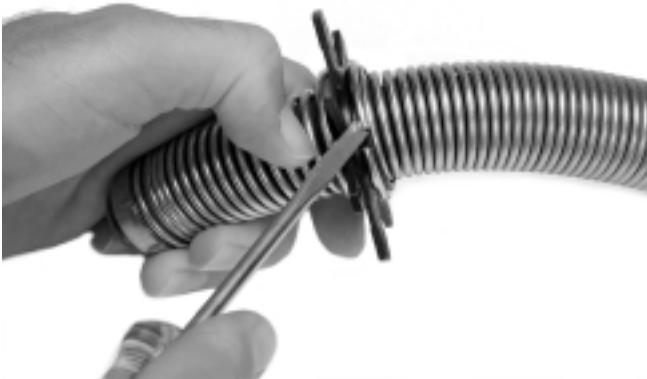
Figure 23 – Place flat tip of screwdriver between c-ring and base of spike and pry c-ring out of groove.
