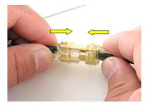
2. Grasp the connector locking sleeve with a pair of long nose pliers and push it back (away from the termination) and over the connection between the cord and FleXmitter.
