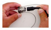
2. Unscrew and slide back the transmitter locking sleeve.
