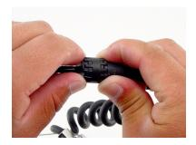
8. Push the female connector through the camera locking sleeve.
