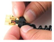
4. Push the cord connector into and through the back of the locking sleeve.
