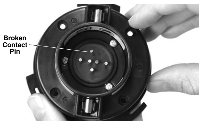
Figure 12 – Broken Contact Pin
