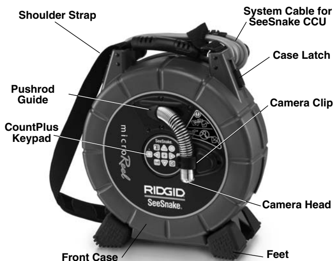
Figure 1 – Front View (SeeSnake Configuration)
