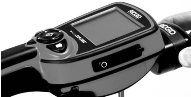
Figure 14 – Raccordement du moniteur microEXPLORER
