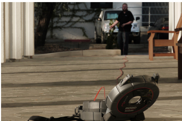
Figure 2 – Straightening the push cable
