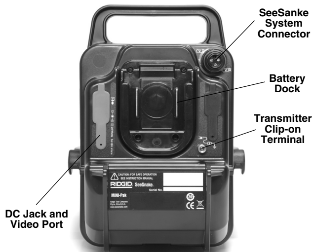
Figure 6 – DVD Pak Connections
