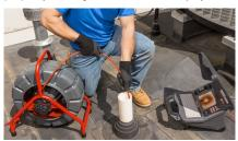
Lay the Mini Pro on its back for greater stability, particularly when on a rooftop, overhead entry, or hillside.
