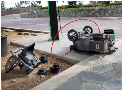
Use the pull handle as a kick stand when performing an inspection on a rooftop, hillside, or in a location that requires overhead entry.
