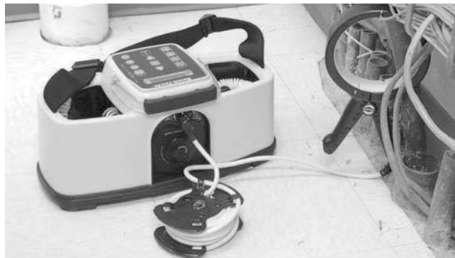
Figure 12 – Inductive Clamp Attached to a Conductor
