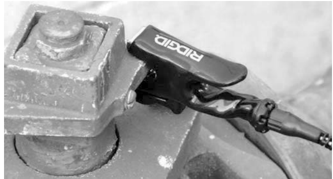
Figure 8 – Connecting Cable Lead To Target Conductor.
